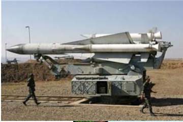
S-200 Angara (SA-5) Strategic Level SAM, operates from fixed sites Radar guided missiles Range: 300 km Source: Stock image
