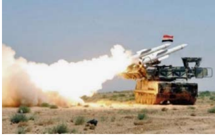
9K37 Buk M1-2+M2 (SA-17) Operational Level SAM, mobile or fixed site Radar guided missiles Range: 30 km Source: SANA
